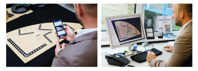
For production of a non-rectangular sheet (shape, free form), glass processors frequently receive a hand drawing or a wood, chipboard, or cardboard template from the customer. However, modern production using a CNC machine requires digital data in order to define these shapes.
