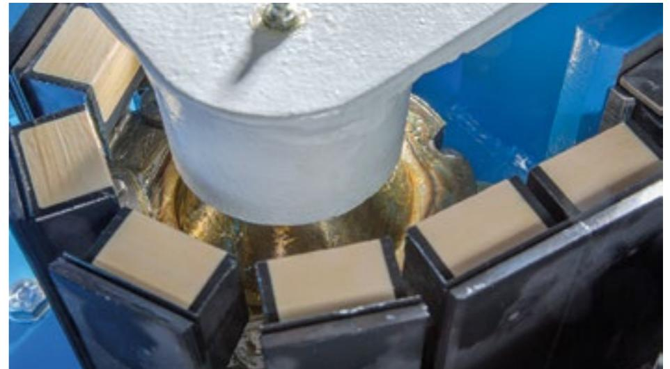
Coolant is applied via efficient water manifolds ensuring a precise and abundant supply of water on the bands of the grinding wheels. This system also allows easier cleaning operations and makes it easier to change the tools.
