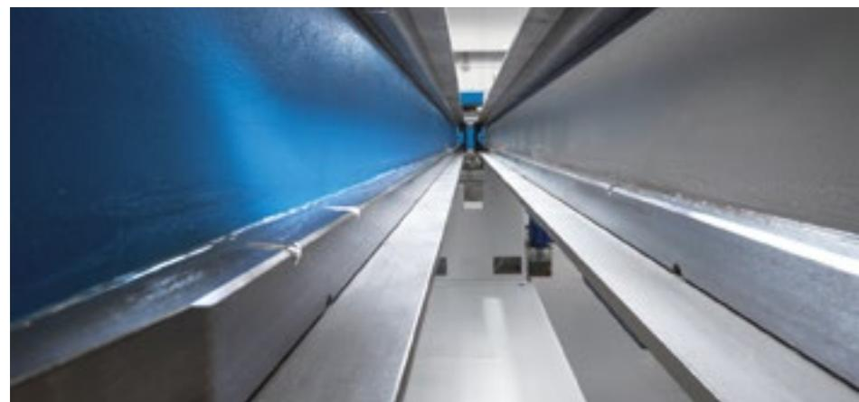
The main conveyors slide on rectified steel guides automatically lubricated by a film of oil and adjustable. This system guarantees maximum precision and extended lifetime.
