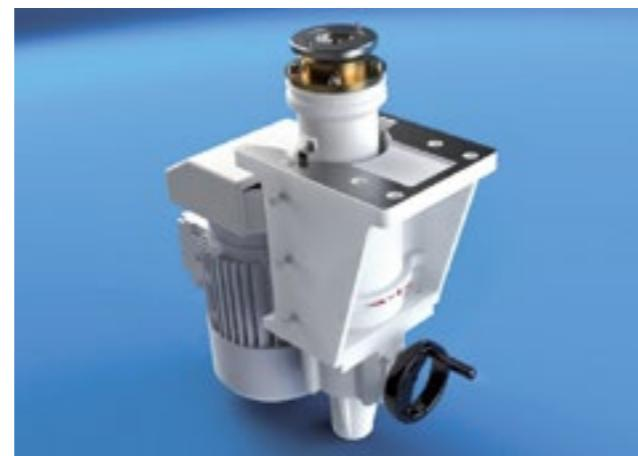
Fully cast iron spindles with separated motorization and belt drive transmission, coupled with the structure of the conveyor through solid cast iron boxes. This compact structure ensures minimum vibrations over the whole lifetime of the machine. Automatic adjustment of the front arris according to the glass thickness.
