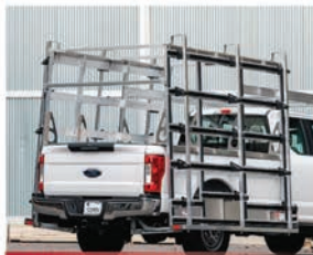
Exterior Glass Rack
